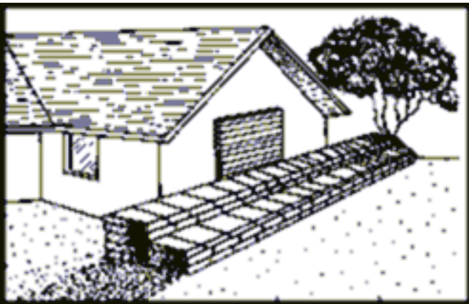
Fig.5 SANDBAG STACKING AGAINST BUILDINGS
